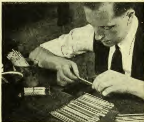
Forming the constriction in the bore
